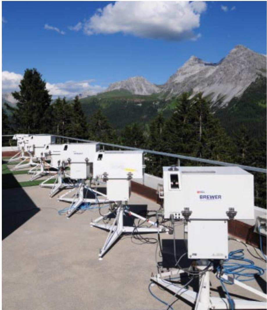
UV radiation and Ozone measurement inter-comparison of Brewer spectrophotometers at the Lichtklimatisches Observatorium of MeteoSwiss in Arosa
